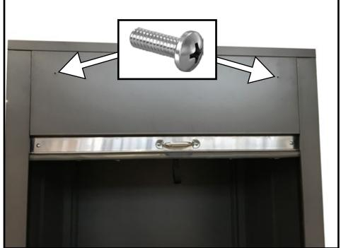
Attach header by engaging keyholes to screws then tighten both screws
