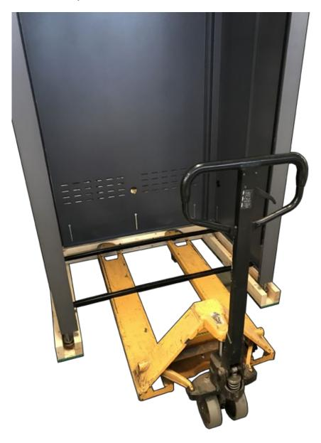
8 Slide wood base free from shroud and dispose of wood parts
