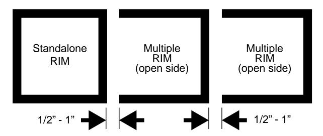
*NOTE: Per Kroger, ensure RIM is NOT closer than 2" to any surrounding bollard, column, or other structure*
