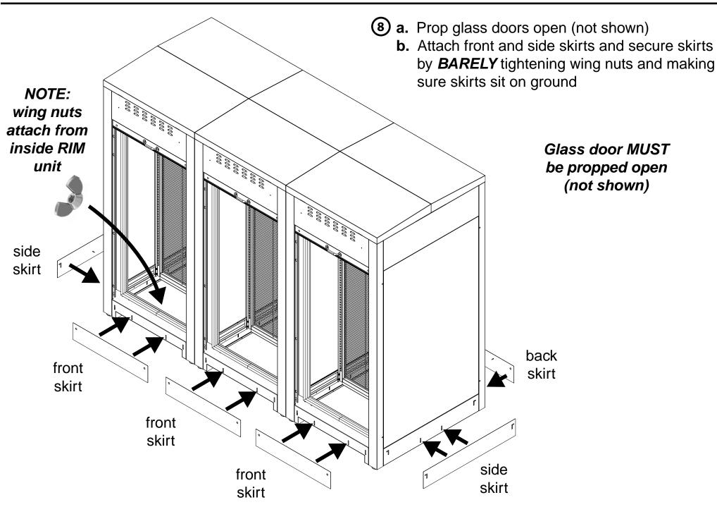
Attach each corner skirt so one stud goes into the L shaped slot on the side skirt
