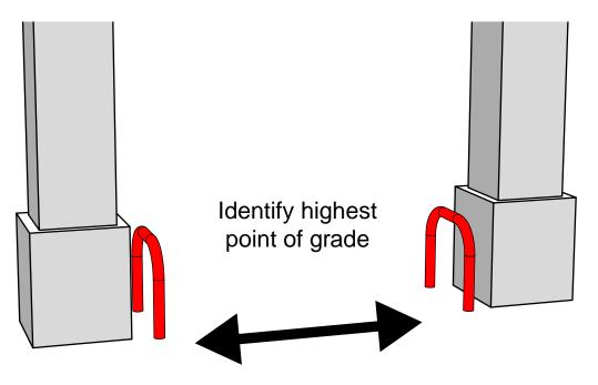
**(6)** Starting with highest grade RIM, adjust levelers higher as little as needed to level unit
