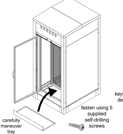
a. Close glass door and install 2 supplied machine screws on each side of RIM and leave screws loose temporarily
