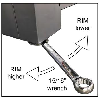
NOTE: For each RIM, adjust levelers as needed, but try to keep RIM to max of 1.5" from the ground
