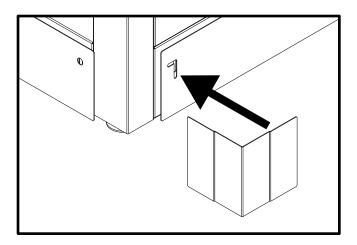
b. Align second stud through hole on front/back skirt, then wing nuts can be attached and BARELY tightened
