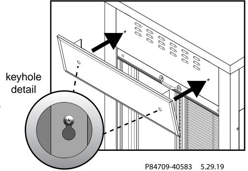
Place 4 plastic hole plugs in unused connection holes on left end and right end of RIM units
